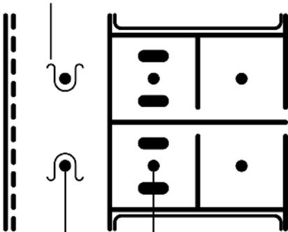
Click the WaterUps® Joiner into the locking holes on the WaterUps® Cells to secure the reservoir liner.
