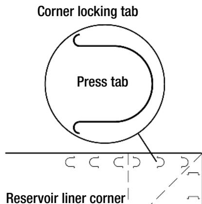
Lock the tabs into the slots in the last layer of the folded liner to secure the corners in place.
