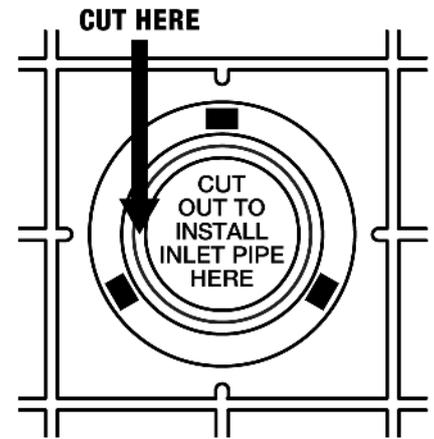
The three tabs on the bottom of the water inlet pipe must lock into the three holes in the tops of the WaterUps® Cell. Apply some pressure to the inlet pipe as you insert it, until it clicks into place in the WaterUps® Cell.
