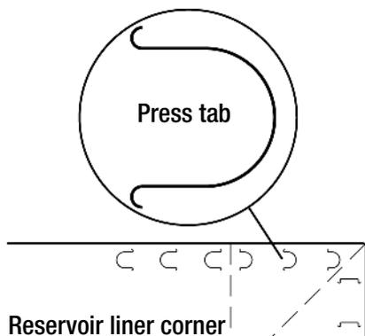
Lock the tabs into the slots in the last layer of the folded liner to secure the corners in place.
