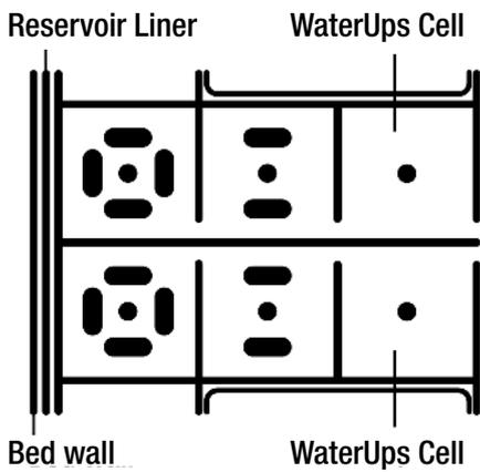
Fold the reservoir liner flap down over the WaterUps® Cells and fold the flap locking tabs back under the reservoir liner to expose the Joiner locking holes in the WaterUps® Cells.
