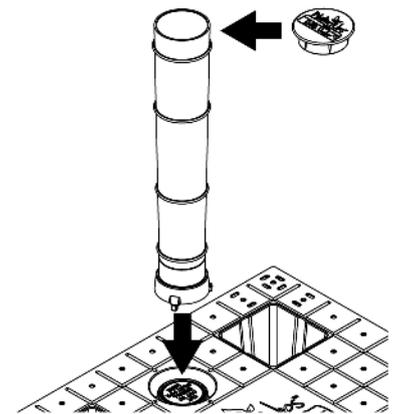
Once the inlet pipe is fitted, place the cell into the last remaining spot in the reservoir liner.
