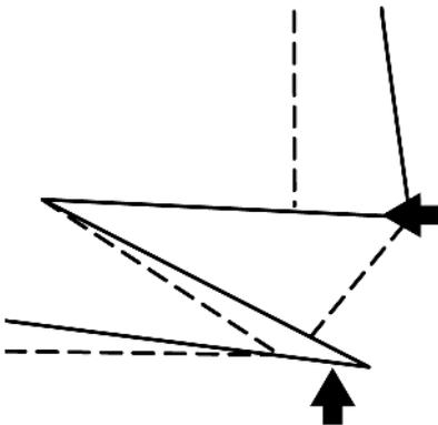
To secure the corners push the three locking tabs through the first two layers of the reservoir liner.
