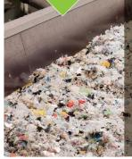
After cleaning and cutting the assorted raw material is processed into granules for injection processing
