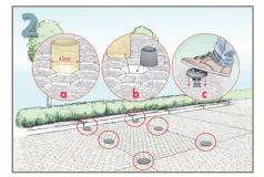
Detail (a) The selected cells should be kept without gravel, whilst the surrounding cells are filled up to the top of the sheet. A 42 mm tube can be used for achieving this.
